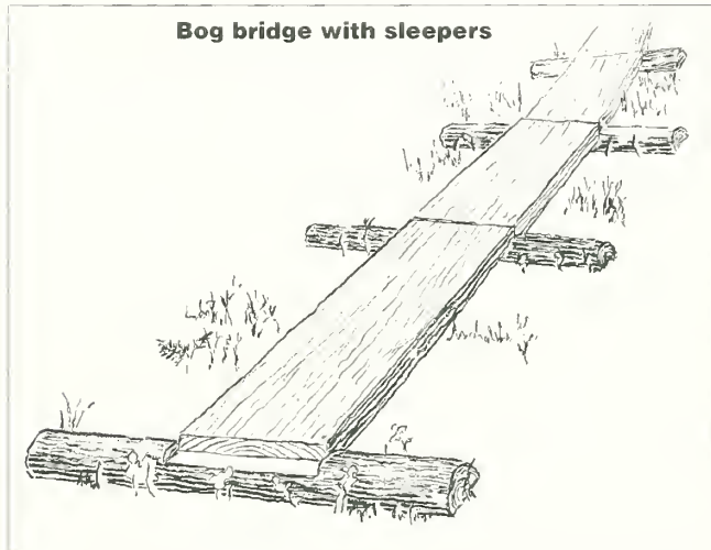
Figure 50—A simple bog bridge with sleepers. This common structure is also called a single-plank boardwalk in coastal Alaska.
